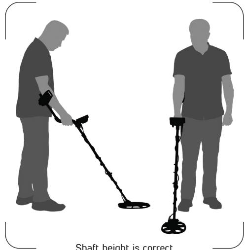
Shaft height is correct
