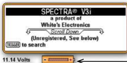
Battery Voltage Reading
