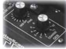
These two GEB controls FINE & COARSE adjust or balance the interference from ground mineralization. FINE makes minor adjustments, COARSE major adjustments. They are only operative when the FINE control is set clockwise from the OFF position.
