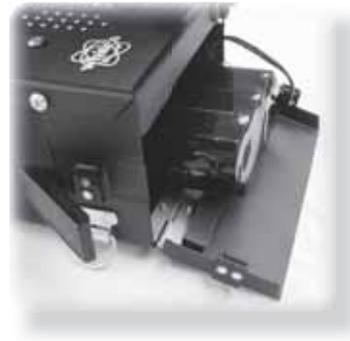
The Pulsescan TDI Pro uses a rechargeable Lithium Ion Battery pack as the power supply. This type of battery is required to supply the high current levels while weighing much less than other battery packs that have similar power characteristics. It supplies a nominal voltage of 14.4 volts and approximately 500 ma of current during use.
