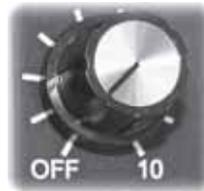
The ON/OFF GAIN control turns the Pulsescan TDI Pro, ON (clockwise) and OFF (fully counterclockwise) and selects the range at which the detector will hear a given target. Gain increases or decreases the amplification of the receive signal determining both how deeply the Pulsescan TDI Pro will hear a target (in ideal conditions) combined with how it is influenced by ground and external interference (in less than ideal conditions).
